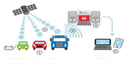
The Gobra Telematics solution in the vehicle (1), obtains vehicle trip data and also GPS position (2), which are transmitted via GSM/GPRS/3G (3), to the server at the Cobra Service Centre (4), from where they are made available to the customer via phone or internet (6).
